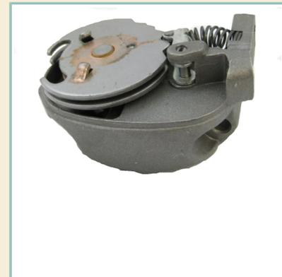
**Cod. 610369M** Selettore cambio Vespa PX (1978) / Gearbox selector Vespa PX (1978)
